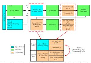
Figure 2 The Functional Block Diagram in the Optimizing Operation of the Simulation Tool for WiMAX Base Station Capacity
